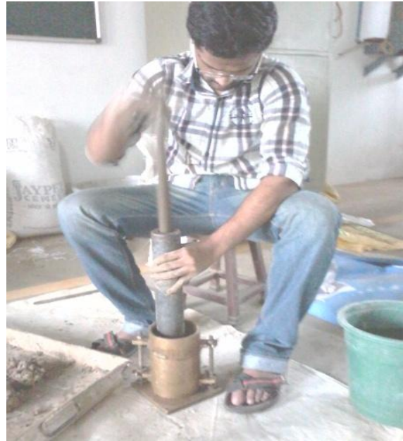
Figure 2 Preparation of mixture by author for compaction test
