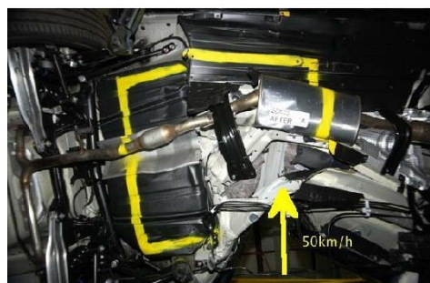
Figure 9. Underside of 50km/h vehicle. The yellow rectangle shows the approximate location of the rear floor area.
