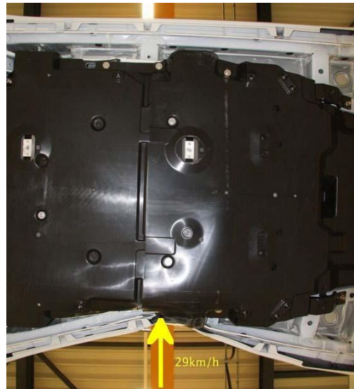
Figure 7. Post crash underside view of vehicle deformation. Battery pack is under the plastic panel at left
