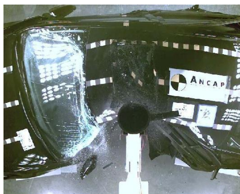
Figure 8. ANCAP research crash test at 50km/h
