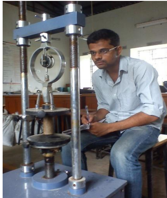
(a) Sample for UCS test (b) Author performing UCS test
