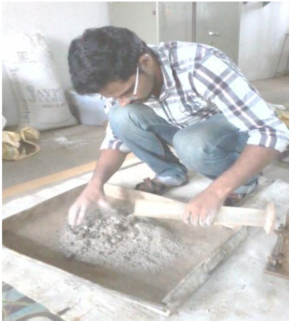
Figure 2 Preparation of mixture by author for compaction test
